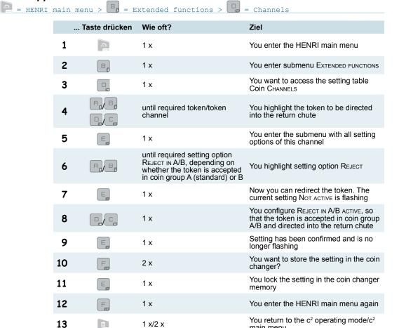
**3** Disconnect and reconnect the coin changer twice. The new setting has also been stored in the changer interface.
