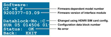
Fig. 17: Interface module diagnostics OK
