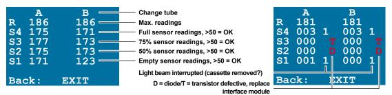
Fig. 24: Filling level sensor diagnostics OK
