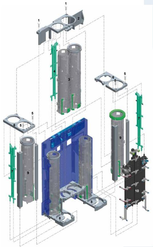
Fig. 12: Assembly plan for coin cassette
