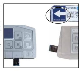
Fig. 2: Inserting SIM card
